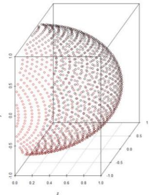
View factor calculation: using equal solid angle ray distribution
