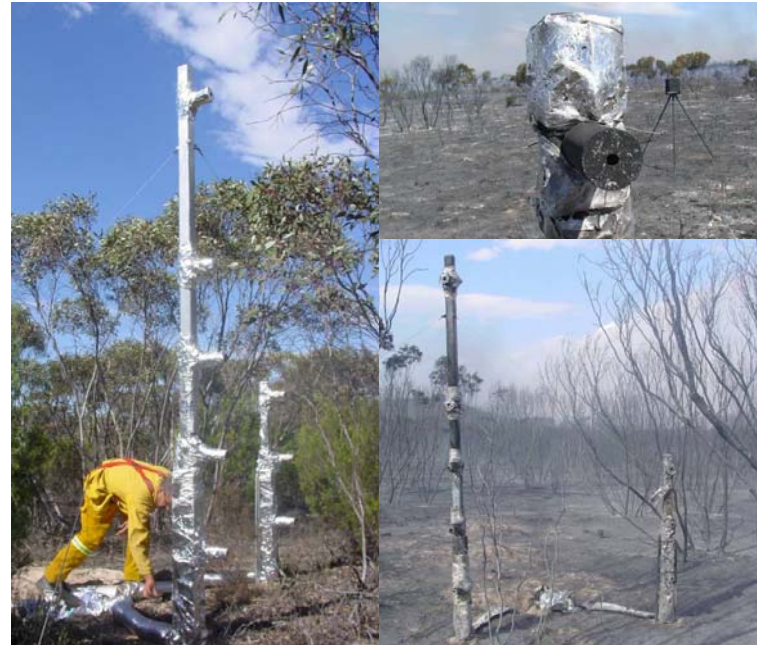
Setup and post-fire view of instrument towers.
