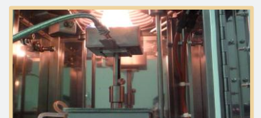
Fuel burning in mass-loss cone calorimeter
